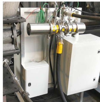
Fig. 2 : Insittec with gantry and enclosures installed on the production line
